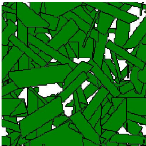
Fig. 2: Simulated microstructure of \text{Si}_3\text{N}_4 by microstructure-property-simulation using the finite element method of the Fraunhofer-Institut für Silicatforschung ISC with sustained, hexagonal \beta -crystallites without preferred orientation [1]
